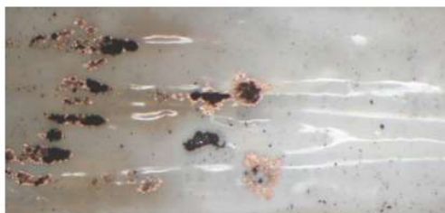
Figure 8. Copper dendrite formation observed on the separator due to repetitive overdischarge.
